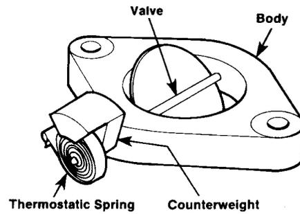
**Thermostatically-controlled heat riser**
