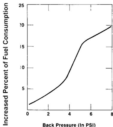
Fuel consumption increases with an increase in back pressure.
