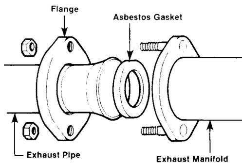
Manifold connections to the exhaust pipe
