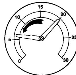
Vacuum gauge reading will drop if a restriction exists.
